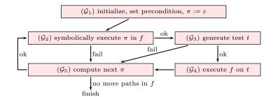
Fig. 3. The PathCrawler test generation method
